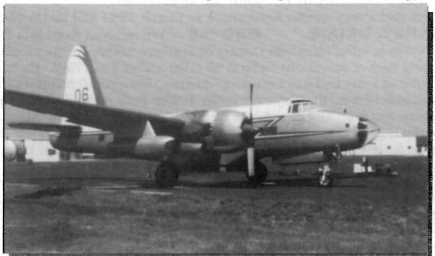
One of Neptune's P2V-5 air tankers sitting at the Missoula jumper base in 1998. This is Tanker 06. Tanker 08 was a newer version with two 3,500 h.p. engines. All of Neptune's air tankers have Westinghouse J34 turbojets under the wings.
