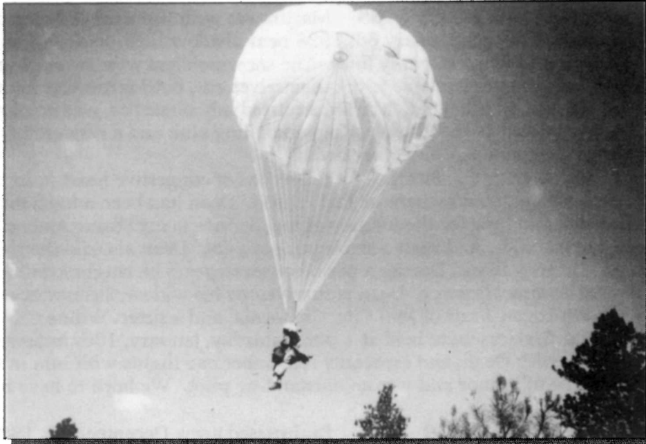
A Missoula jumper descending to a fire in Western Montana during the summer of 1995. He is using an FS-12 parachute. This is a 32 foot, flat, circular, multiple porosity chute. It took the place of the FS-10.
