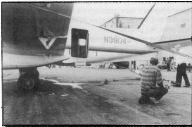
A Bandeirante's static line cable and anchor being tested for strength at the Missoula County Airport by members of the MTDC in the 1980's.
